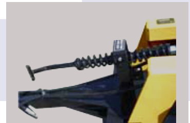
Self-leveling, spring cushioned hitch with hand crank
